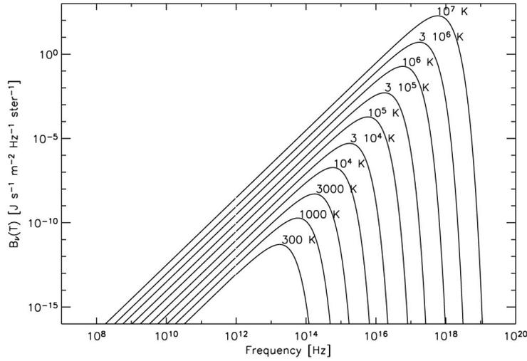
**Figure 2.2** : Spectrum of blackbody radiation at various temperature (from Kraus J.D. 1966)
