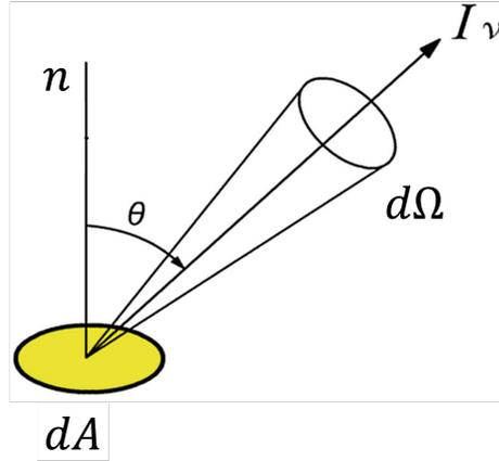
**Figure 2.1** : Geometry for obliquely incident rays
