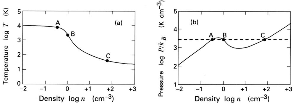
**Figure 2.8** : Left : Equilibrium temperature versus number density ; Right : equilibrium pressure versus number density.
